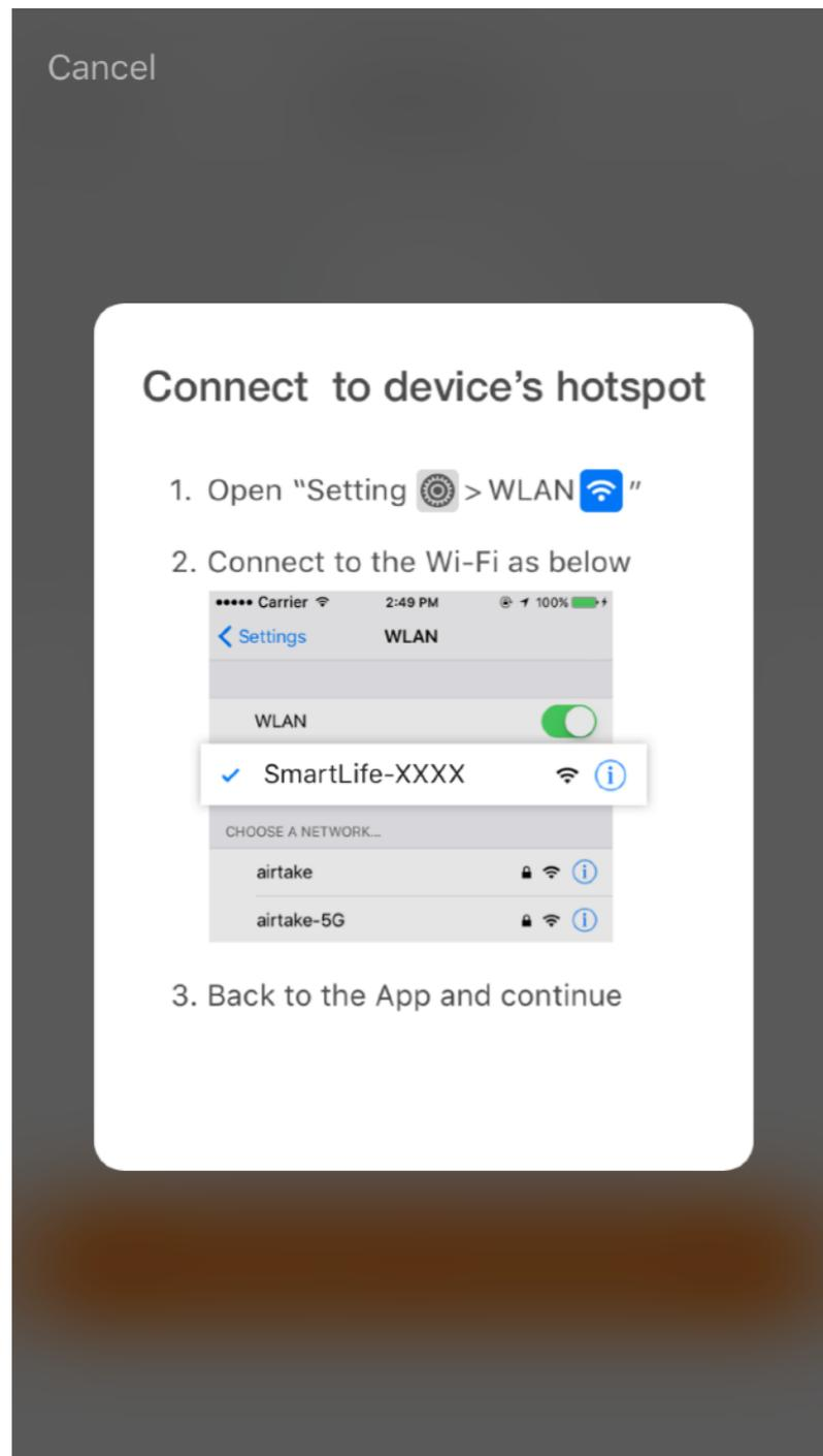
For AP mode, connect to the Wi-Fi hotspot named "SmartLife", as shown in the picture
